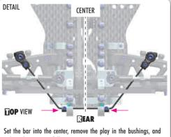
Set the dar into the center, remove the play in the dusnings, and tighten the setscrews fully.
